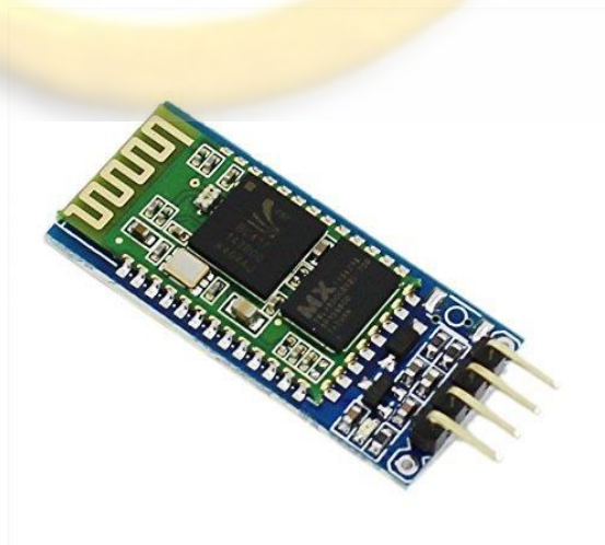
Gambar 2.7 Modul Bluetooth HC-05
