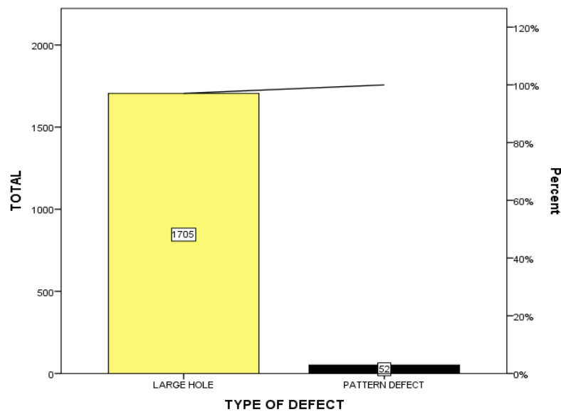
Figure 2. Pareto diagrams for each type of product defect type 04G22 Source: Processed Data, 2020
