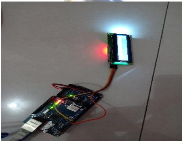
Fig.6 Implementation of LCD Module
